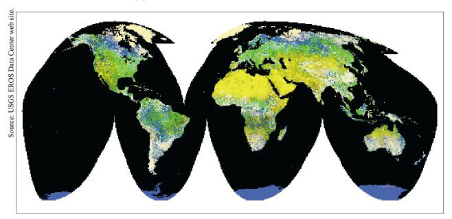
AVHRR (Advanced Very High Resolution Radiometer) imagery such as this is useful for global and regional scale land cover change and environmental monitoring, and for selected meteorological and climatological applications.
