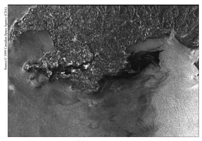
A Radarsat Synthetic Aperture Radar (SAR) image picks up an oil spill along the coast of Wales. The only known instance of remote sensing imagery being used in a compliance verification mode was the case of an oil spill in the straights of Malacca near Singapore under the MARPOL convention.
